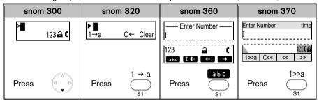
Result: The input mode has been changed to lower case. The display shows:
