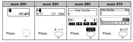
**Result:** The input mode has been changed to *numeric*. The display shows:
