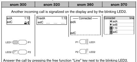
**Result:** The first active call on the free function "Line" key P1 is placed on hold and the 2<sup>nd</sup> incoming call on the free function "Line" key P2 is accepted. This is indicated by a slowly blinking LED1 and a permanent lit LED2. Additionally a tone sequence can be played to remind you of the waiting call.
